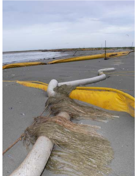
Boom washed up on Elmer's Island, LA. Both white sorbent boom, which is designed to absorb oil, and yellow harbor boom are visible. / Mike Parr, American Bird Conservancy
