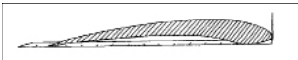
Fig. 3. Wing chord as measured with a wing ruler, without flattening or pressing down on the wing.
